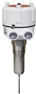
A vibrating rod features a single probe design that prevents material from bridging and giving a false signal.
