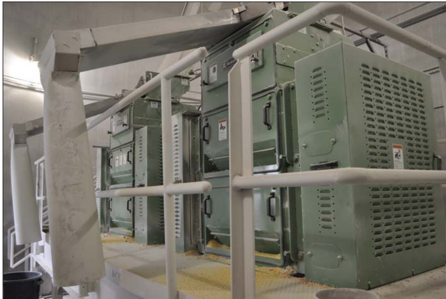
A pair of 45-tph Roskamp Champion roller mills grind whole grains prior to sending them to the ingredient bins.
