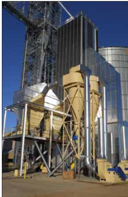
Two new 7,500-bph LMC aspirators remove light fractions from rice.
