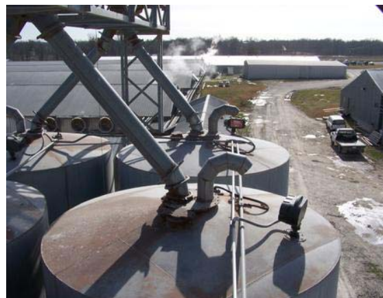
SmartBob II Remotes measuring finished feed bins at Rose Acre Farms in Knob Noster, Missouri
