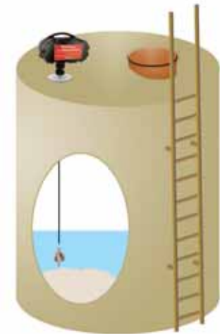
Brine Tank measuring Submersed Solids
