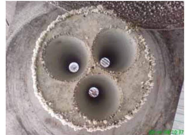
The outside of the unit is coated with dust. The sensors inside the unit are clean and fully functional.
