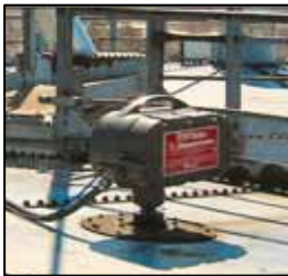
Measuring carbon black in a rubber belt plant
