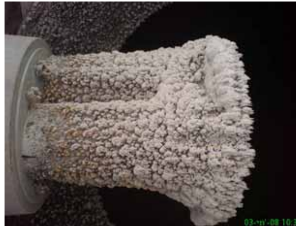
The outside of the unit is coated with dust. The sensors inside the unit are clean and fully functional.
