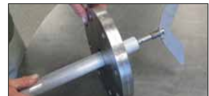
The collapsible paddle "squeezes" shut to insert into the bin and then automatically "pops" open.
