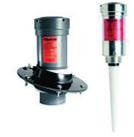
Radar-based devices generate an electromagnetic wave that travels to the material surface being monitored that is reflected off the surface back to the sensor. The calculated distance is based on the length of time it takes the wave to return from the surface.
