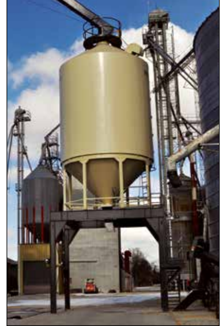
Meridian overhead surge tank is used for loading trucks or as a bypass.
