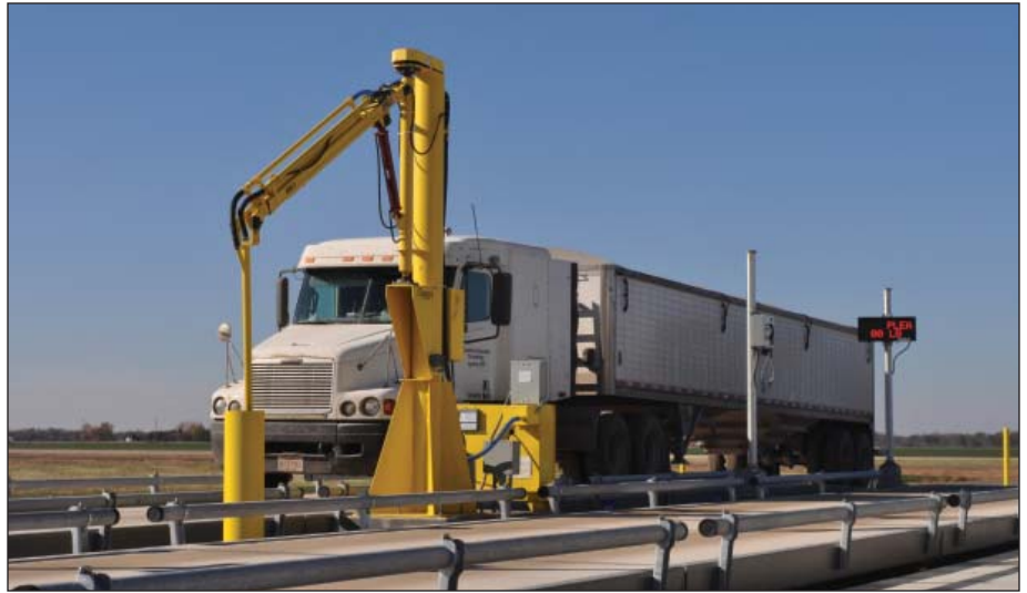
A truck driver moves onto a Mettler Toledo outbound scale after delivering grain. Also visible is the inbound scale and an Apollo truck probe. Ground-level photos by Ed Zdrojewski.
