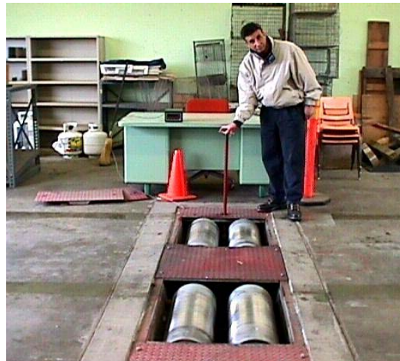
Rollers of a "Rolling Road"
