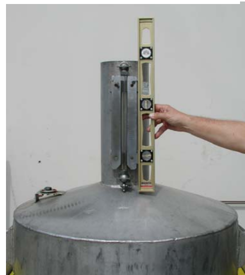
Level Gauge Against Sight Glass
